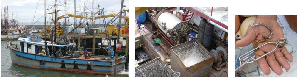
An example of a semi-industrial boat, a long line on a reel with hooks in a crate, and a hook and snap.
